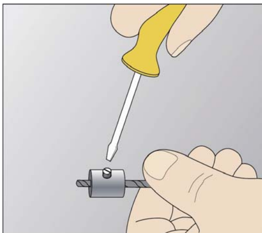
Figure 4A – Setting Drill Stop Collar
